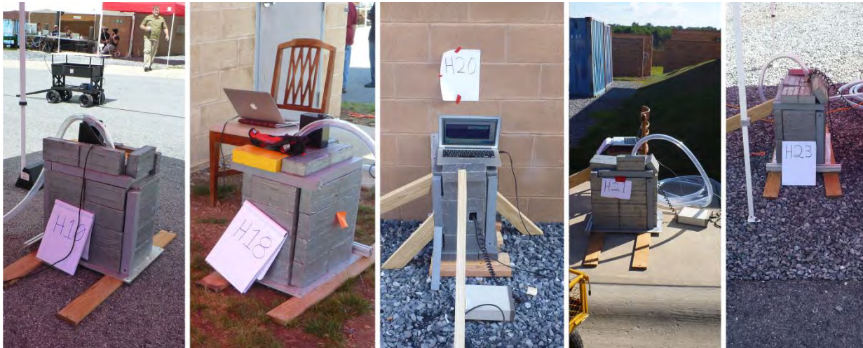
Shielded HPGe detector measuring various sources of background
